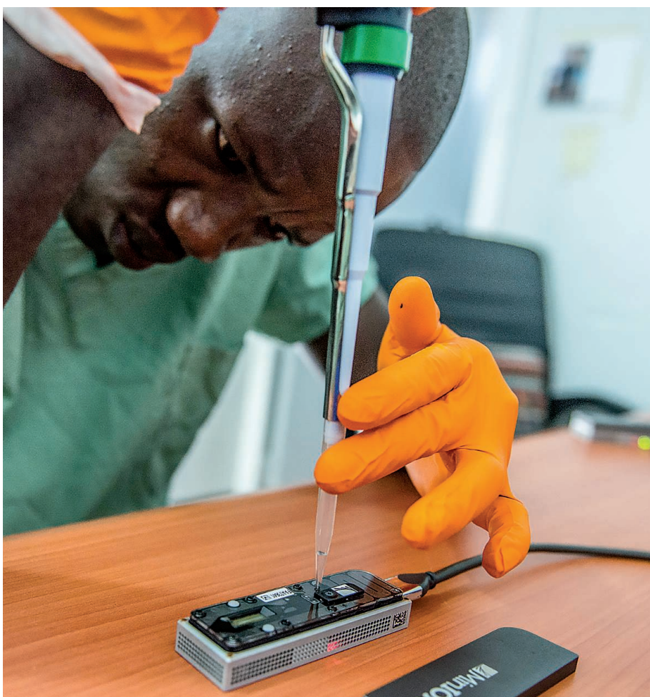
This pocket sequencer, used here during the Ebola outbreak in West Africa, read viral genomes from human samples.
