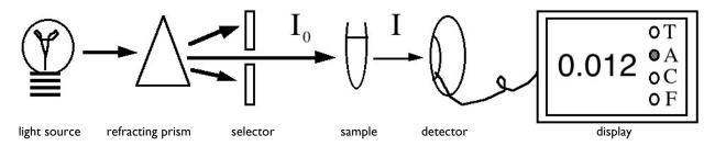
Figure 1. A schematic diagram of the components of a spectrophotometer. The arrows indicate the pathway of light.
