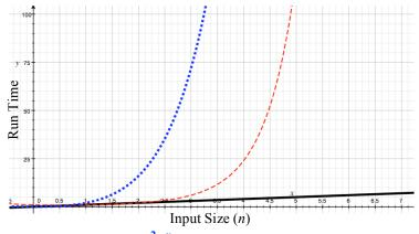
**Figure 2.** Growth functions for O(n!),  $O(n^2 2^n)$ , and O(n). The x-axis represents the input size, *n*, and the y-axis represents run time. From slope analysis of the above figure, it is evident that both algorithms for TSP are extremely inefficient when compared to O(n).
