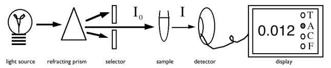
Figure I. A schematic diagram of the components of a spectrophotometer. The arrows indicate the pathway of light.
