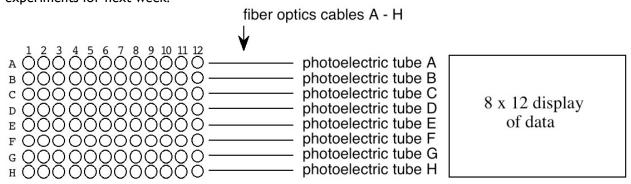
**Figure 2. Schematic diagram of a microplate reader**. Samples are placed in the 96 microwells, analyzed by the eight channel spectrophotometer, and the absorbance data are displayed in the large LED window.
